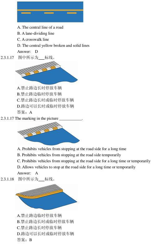
2.3.1.18 The marking in the picture \_\_\_\_\_.
